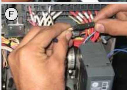
Fig. A: Release Indication Contact kit Fig. B: Removing the existing cover Fig. C: Cover assembly Fig. D: Cover assembly Fig. E: Assembly of coil Fig. F: Assembly of connector Fig. G: Assembly of coil Fig. H: Assembly of connector plug Fig. J: Assembly of connector plug
