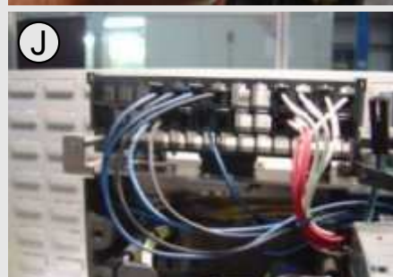
Fig. A: Release Indication Contact kit Fig. B: Removing the existing cover Fig. C: Cover assembly Fig. D: Cover assembly Fig. E: Assembly of coil Fig. F: Assembly of connector Fig. G: Assembly of coil Fig. H: Assembly of connector plug Fig. J: Assembly of connector plug
