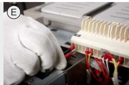
-- Fig. A: Bell Alarm Kit Fig. B: Assembly of Bell alarm Fig. C: Fixing the screws Fig. D: Assembling wire tie Fig. E: Assembly of connectors
